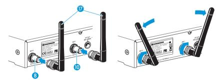
Align the rod antennas upwards in a V-shape.
