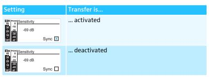
By pressing the symbol button 3, you can transfer the parameters to the transmitters via the infra-red interface (see page 22).
