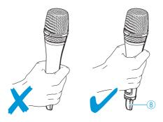
Only hold the radio microphone by its body.
