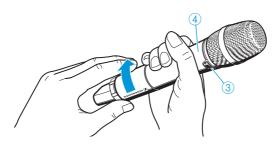
When unscrewing the radio microphone during operation, the muting function is automatically activated. "MUTE" appears on the display panel.
