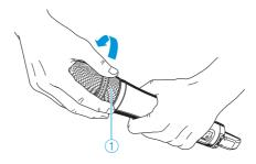
Do not touch the contacts of the radio microphone nor the contacts of the microphone head ①. The contacts can become dirty or damaged if touched.
