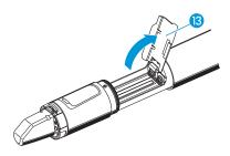
▶ Insert the batteries or the BA 2015 accupack as shown on the battery compartment cover. Observe correct polarity when inserting the batteries/accupack.
